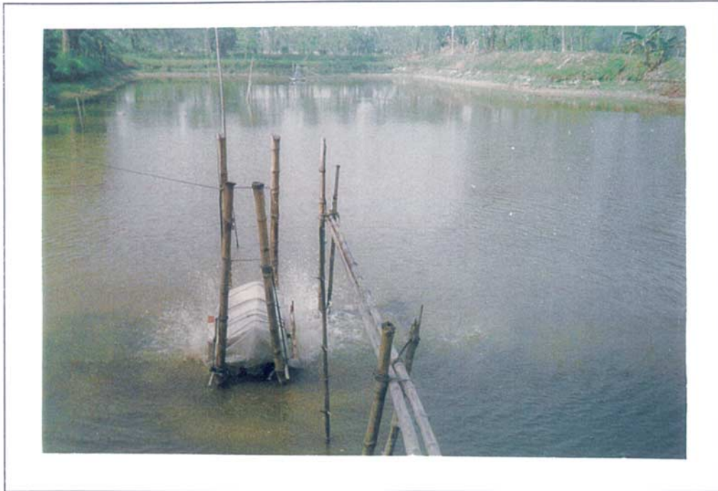
Plate 5.5: An indigenously designed aerator in use by a progressive farmer.
