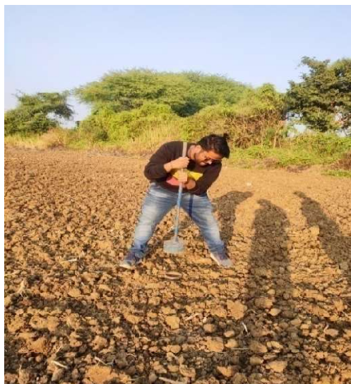
Fig. 3.19 Collection of soil sample by core cutter
