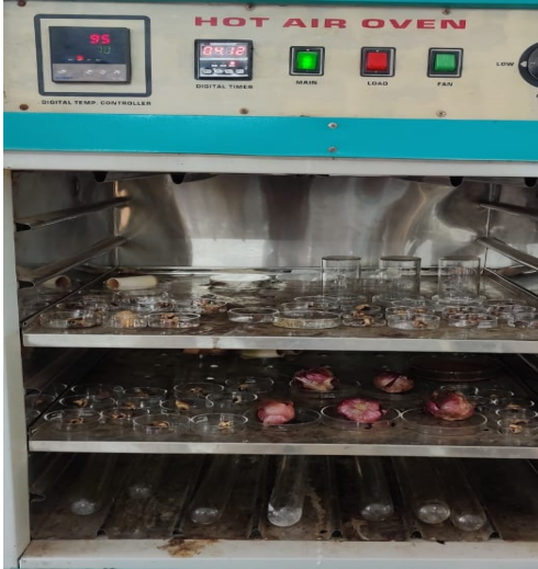
Fig. 3.9 Onion sample kept in electric oven for 24 hours
