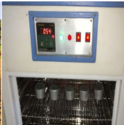
Fig. 3.20 Determination of moisture content of soil sample by oven dry method
