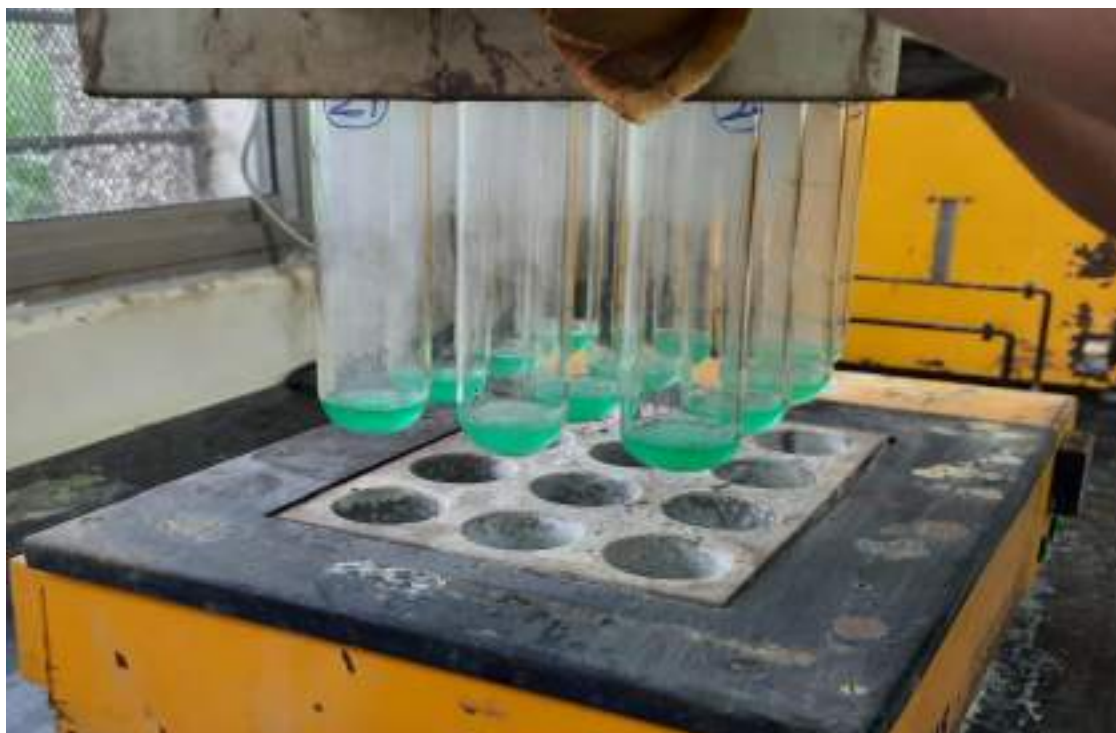
Digestion process during Protein content estimation in mungbean
