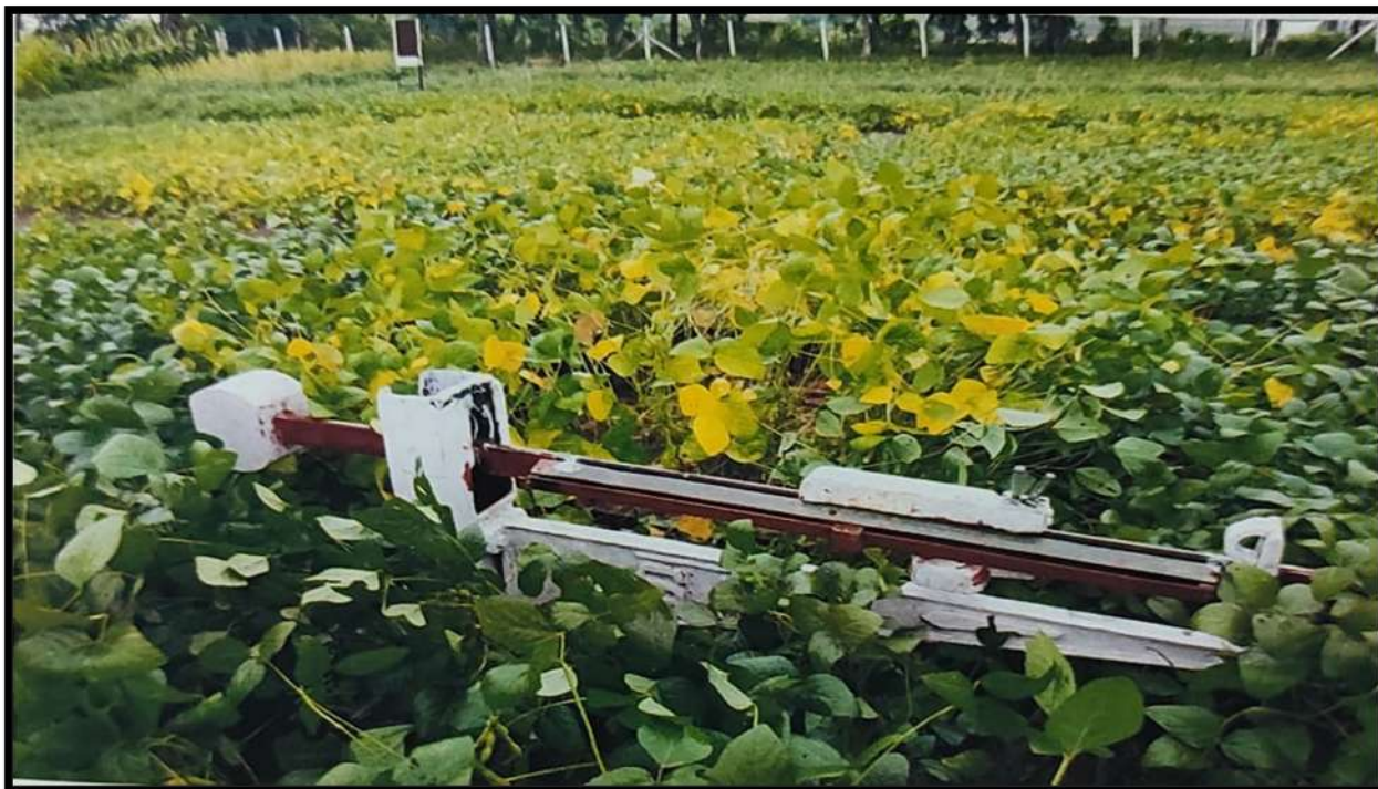
Plate 3.1 Gravimetric or Weighing type of lysimeter containing soybean MAUS-71.
