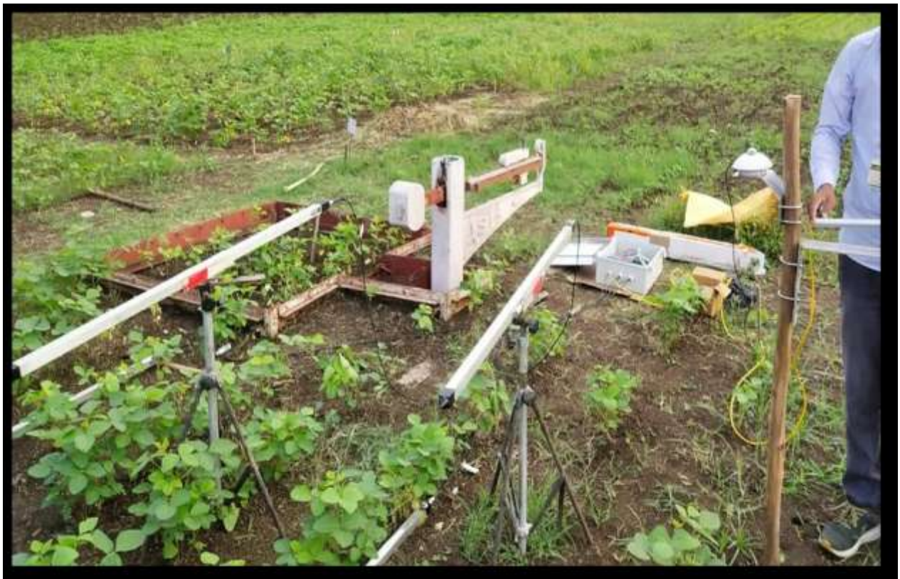
Plate 3.5 Radiation measuring sensors in lysimeter plot.
