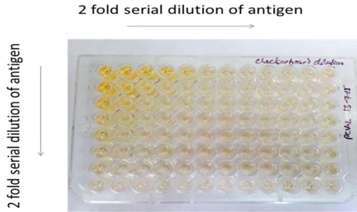
Fig. 12: Optimization of coating antigen concentration by checkerboard dilution method for development of an indirect ELISA
