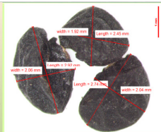
Fig. 1: Onion seed dimensions recorded using microscope - Nikon SMZ 1000 at 2X magnification
