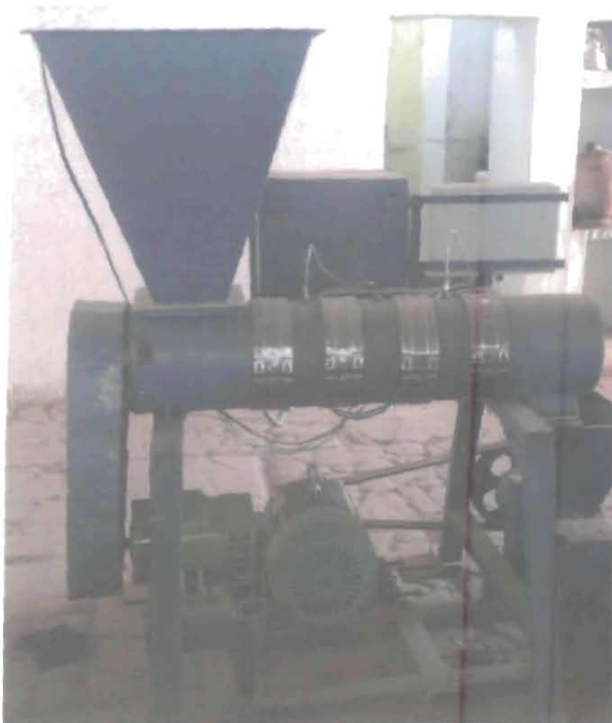
Plate 4.7 Preheater System with mica band heater, sensors and control panel
