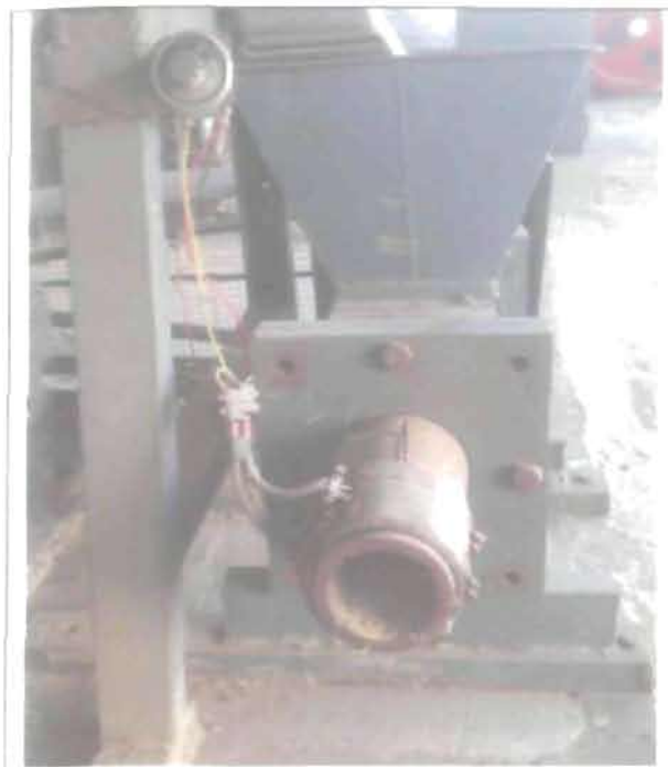
Plate 4.2 Developed Screw Press Briquetting Machine with Heated Die
