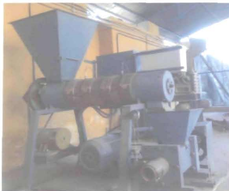
Plate 4.2 Developed Screw Press Briquetting Machine with Heated Die
