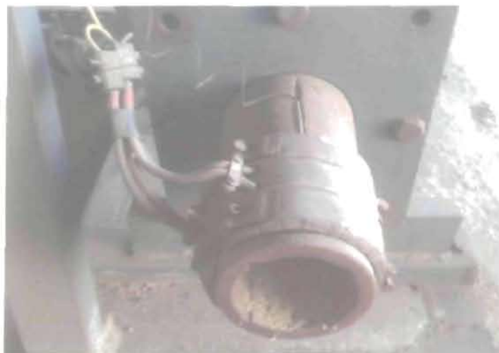
Plate 4.4 Die with Mica band heating system
