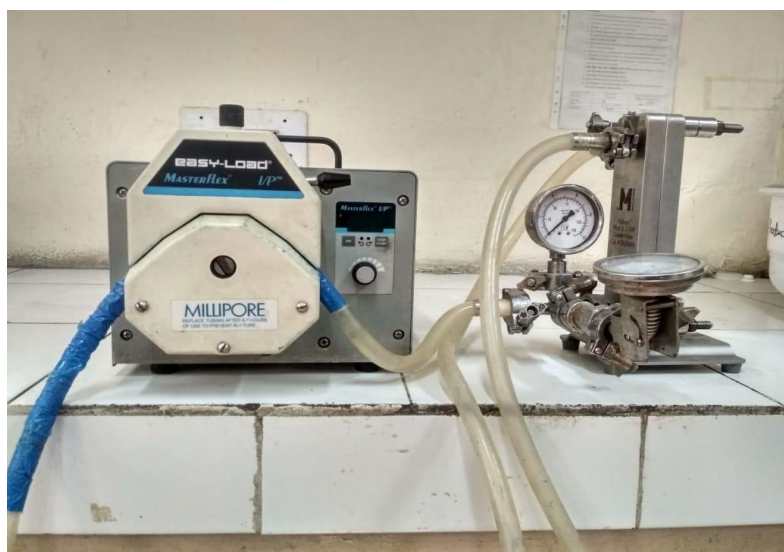
Figure 3.1 Equipment of Ultrafiltration Unit
