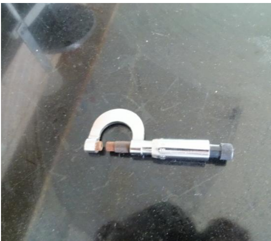
Fig. 3.17: Screw gauge for measuring egg shell thickness
