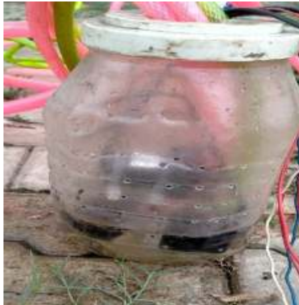
Fig.3.9:- Filter Box (approx. 5 litre capacity)
