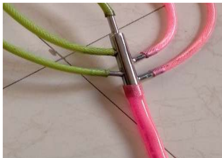
Fig. 3.8:- Outlet pipe for handling the combined discharge of pumps
