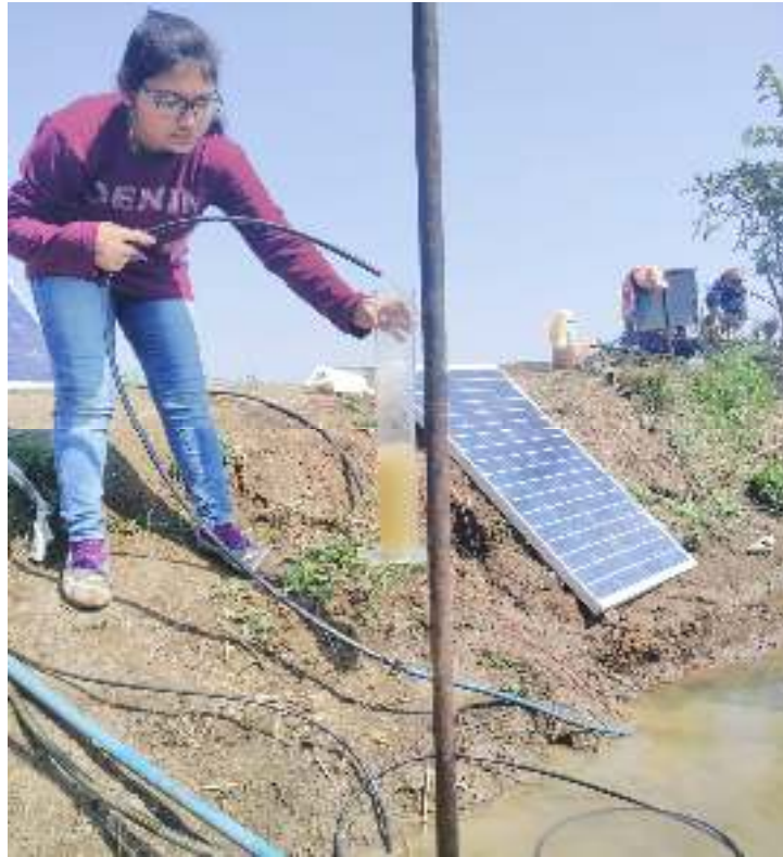
Fig 3.15:- Determination of discharge rate in KVK field using volumetric method
