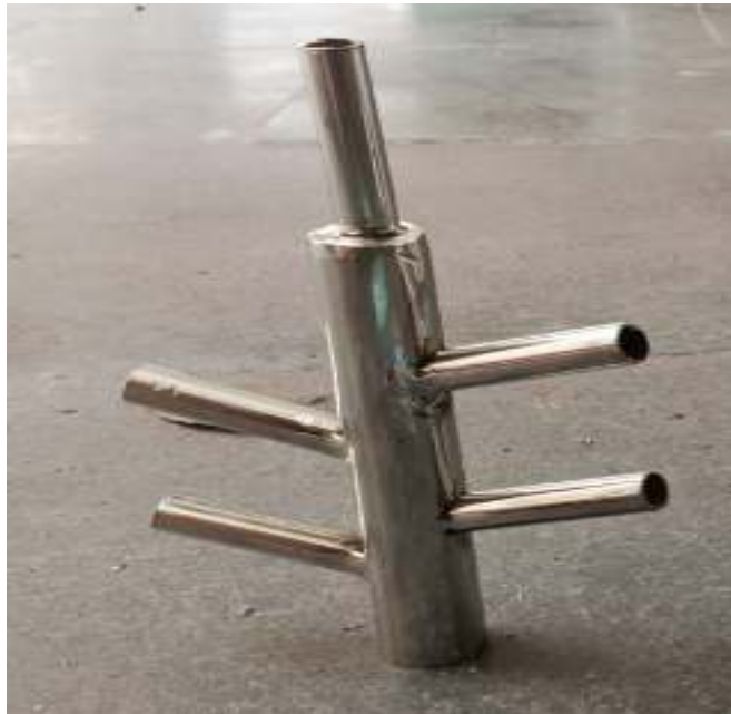
Fig. 3.7:- Jointer for making a parallel combination of pumps
