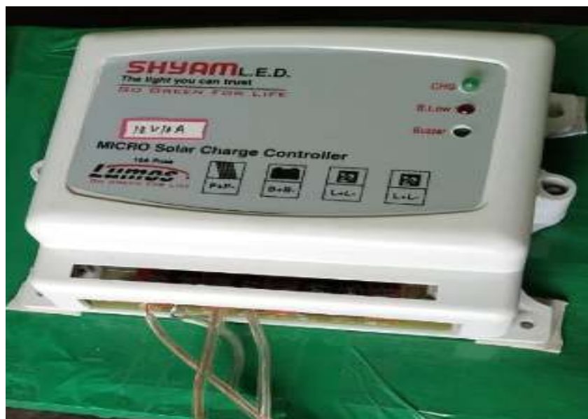
Fig. 3.5:- 12V, 10A Charge Controller Used in this study
