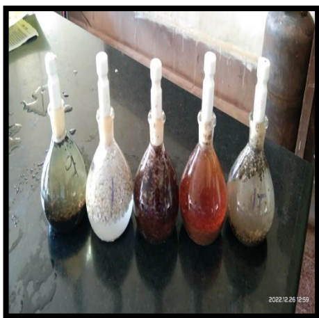
Plate 3.9 Particle density of individual media by pycnometer method
