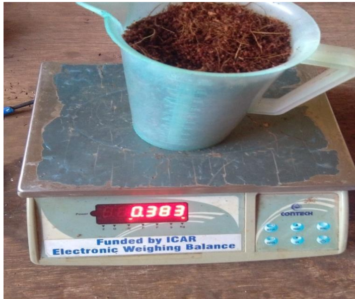
Plate 3.8 measurement of weight of individual media for bulk density
