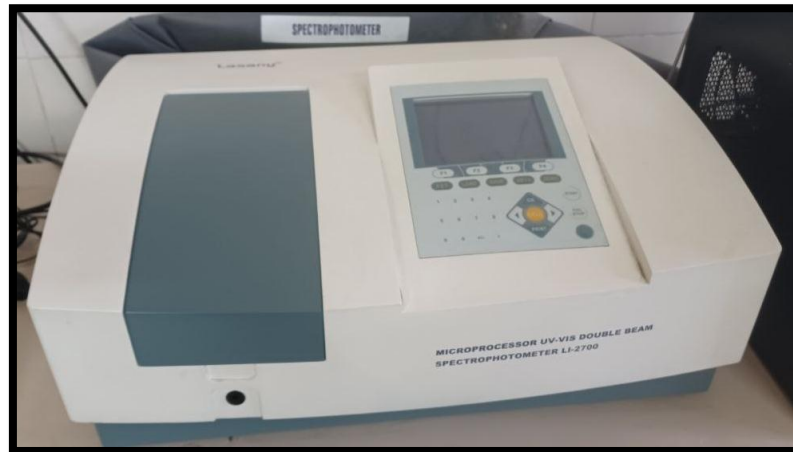
Plate 3.21: Spectrophotometer used for \beta -carotene determination
