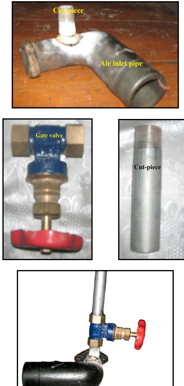
Fig. 4.12 Parts used for engine modification
