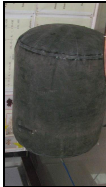
Fig. 4.9 (b) Biogas storage balloon
