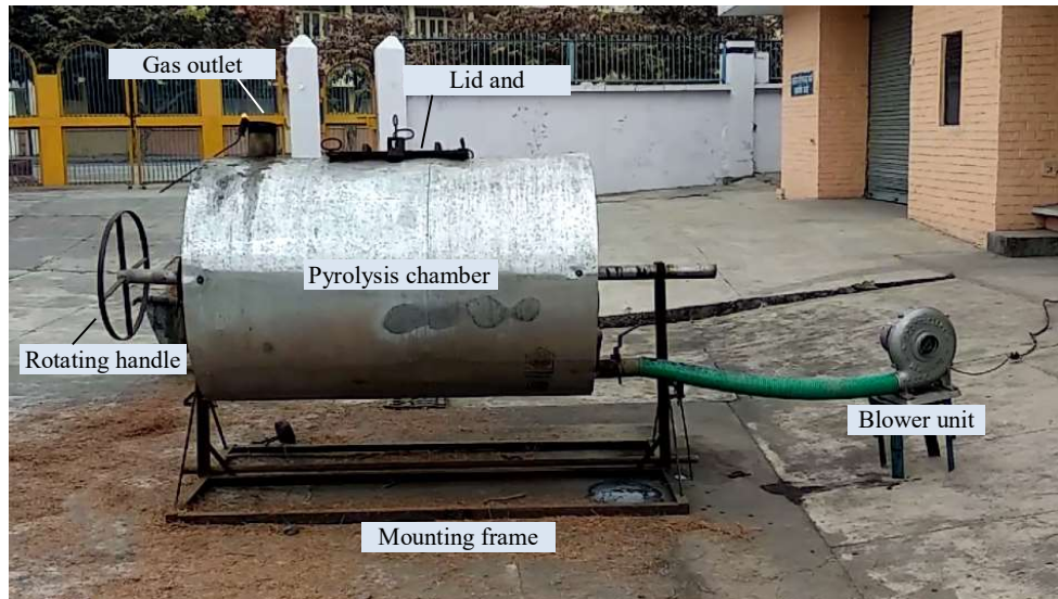
Plate 3.4 Biochar Production Unit (64 kg per batch)
