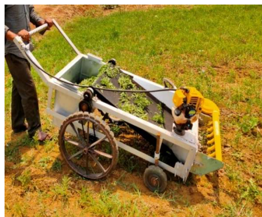
Fig. 3.62: Developed leafy crop harvester
