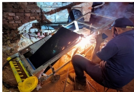
Fig. 3.54: Fabrication of leafy crop harvester
