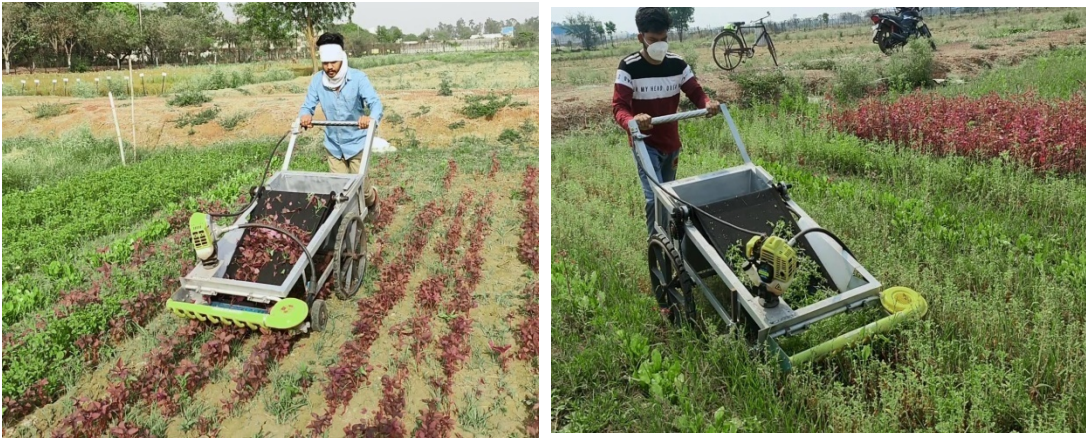
Fig. 3.69: Harvesting of leafy crop by developed leafy crop harvester
