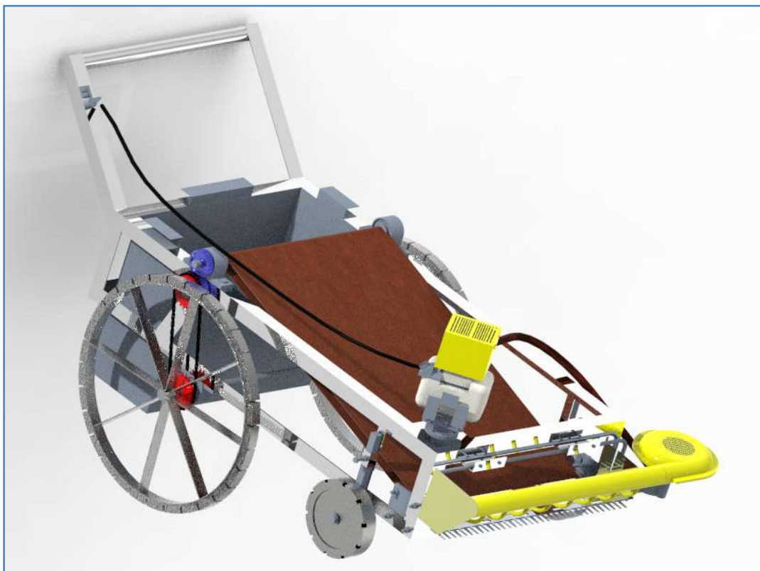
Fig. 3.48: Visual model of leafy crop harvester
