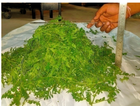
Fig. 3.11: Measuring angle of repose of chickpea by free fall method
