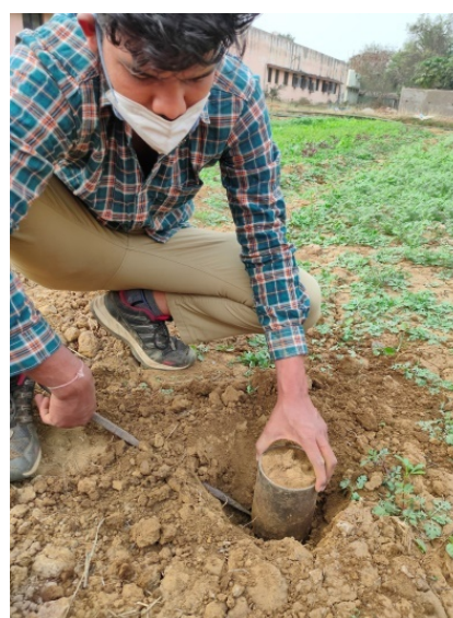
Fig. 3.56: Removing core from the soil
