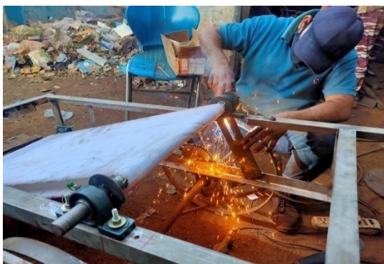
Fig. 3.54: Fabrication of leafy crop harvester
