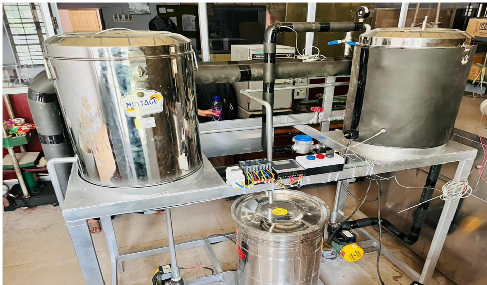
Fig 3.2: Back view of double pipe heat exchanger
