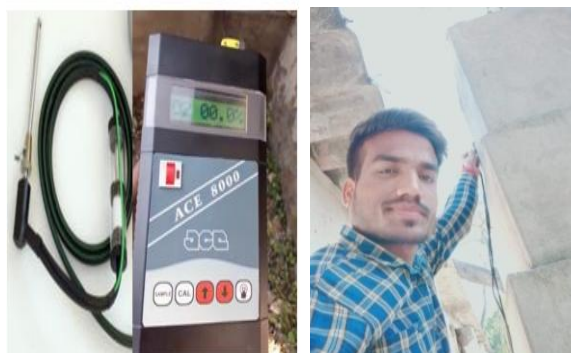
Fig: 3.9: Measuring temperature of the flue gas
