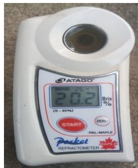
Fig 3.6: Measuring TSS of sugarcane juice
