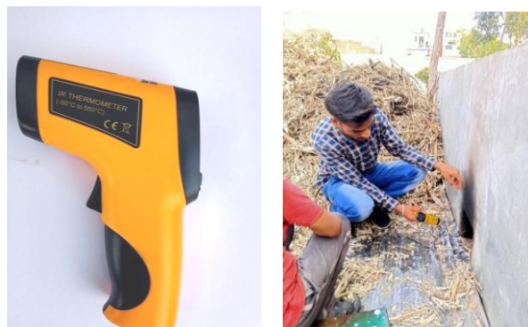
Fig 3.8: Measuring the furnace temperature
