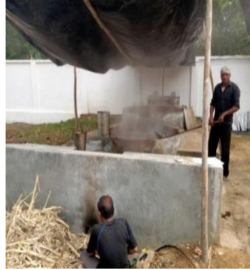
Fig 3.14: Bagasse feeding during jaggery preparation
