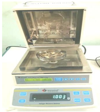
Fig 3.5: Measuring the moisture percentage of bagasse
