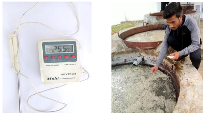
Fig 3.7: Measuring the juice temperature
