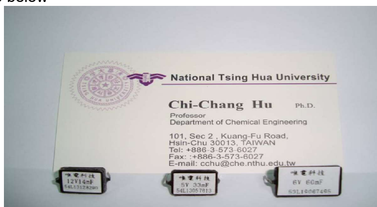
Fig9-Commercial SCmade up of RuO 2 - electrodes
