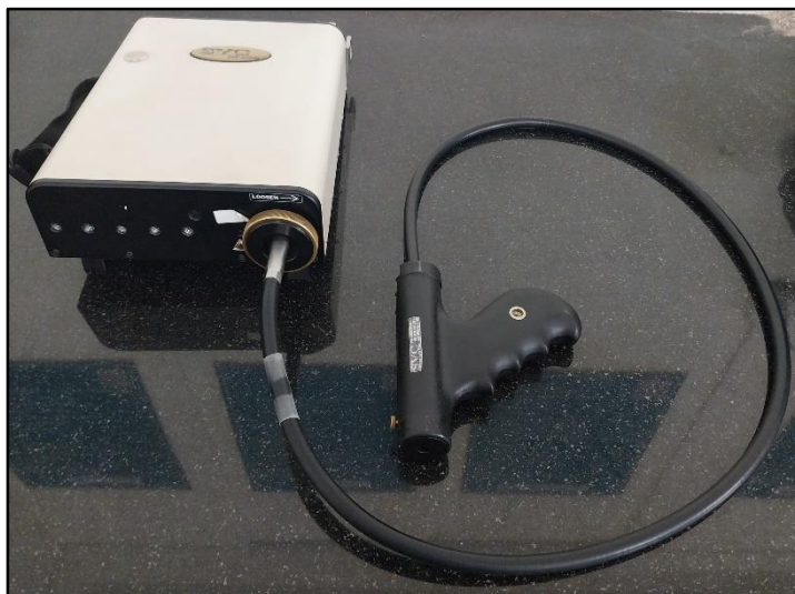
Plate 3.6: SVC (Spectra Vista Corporation) HR-1024i (High Resolution) portable field Spectroradiometer with optical fibre attached.
