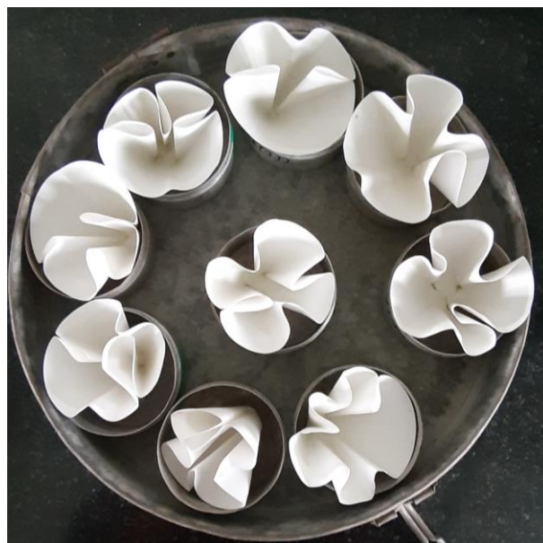
Plate 3.5: Traces of suspended sediment filtered by Whatman paper after oven drying
