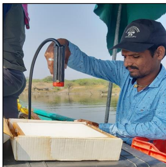
Plate 3.8 Capturing spectral response of reference/ Spectrolon panel
