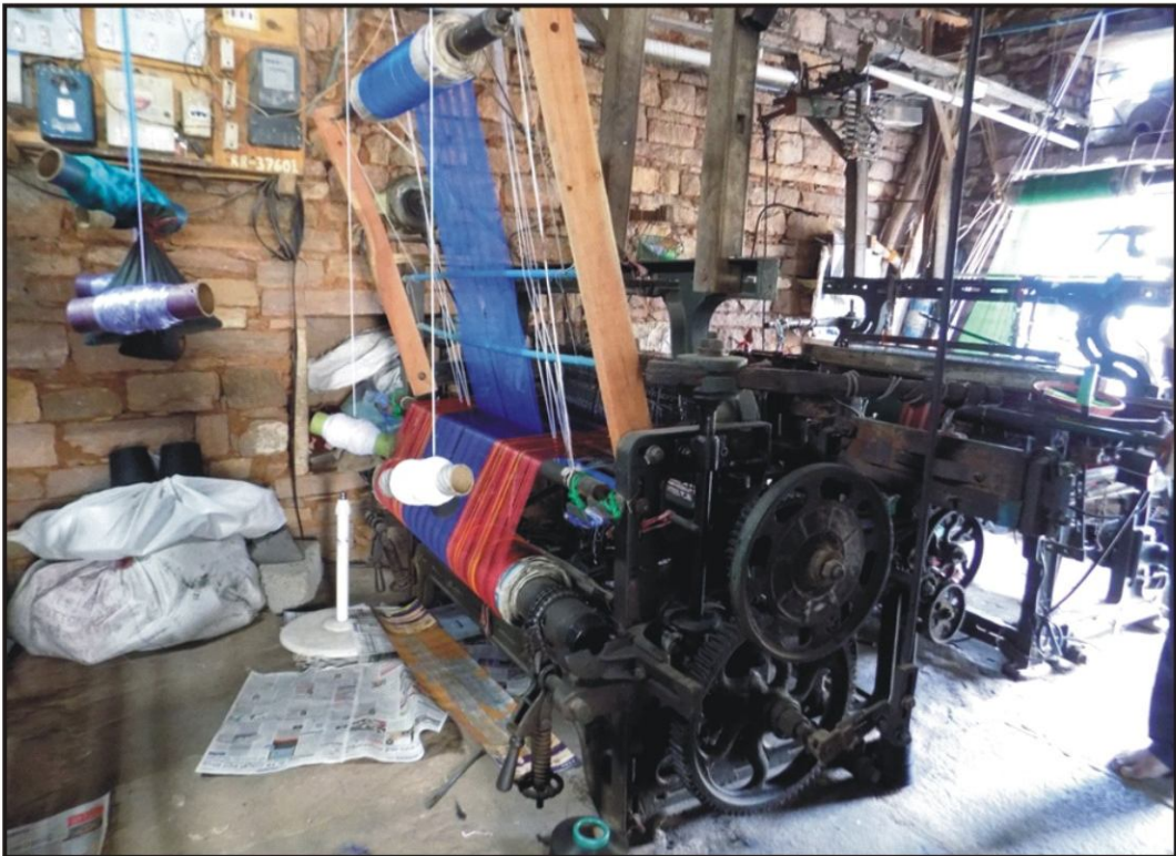
Plate 1. Powerloom attached with extra warp beam
