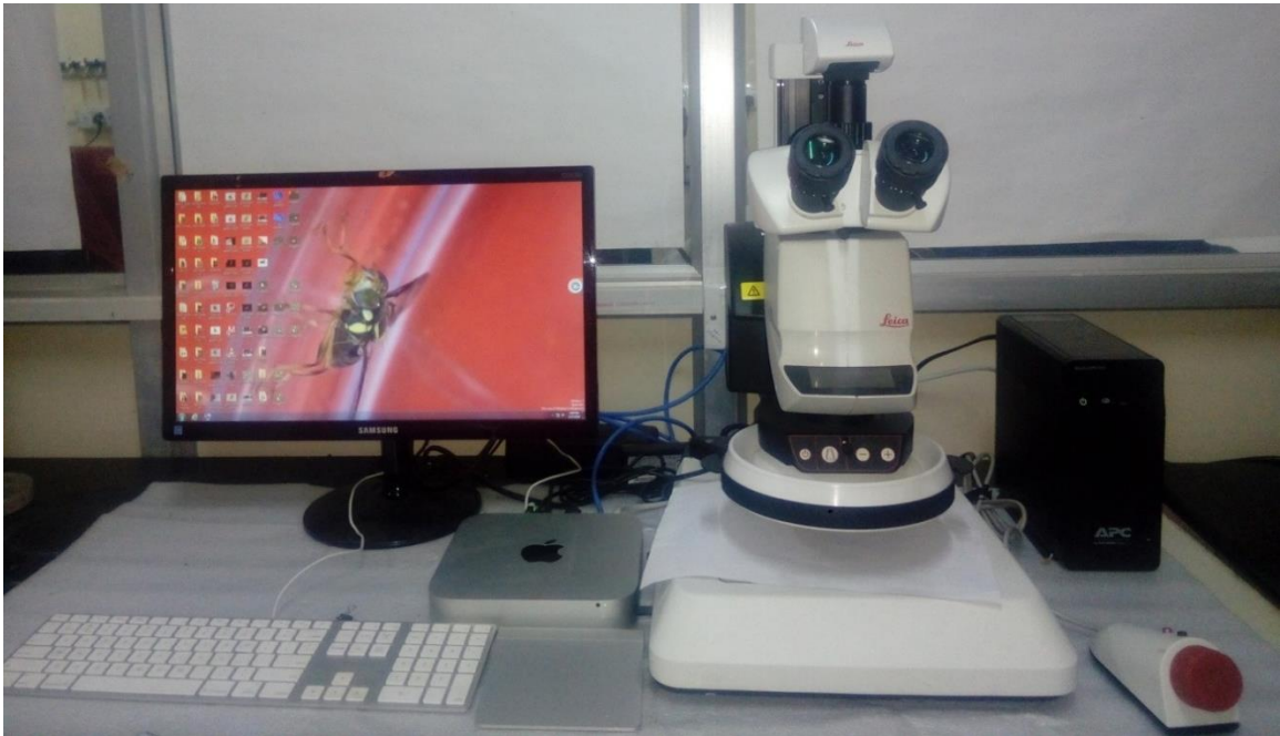
Plate 10. Microscope used for eggs count and sex identification in pupal stage
