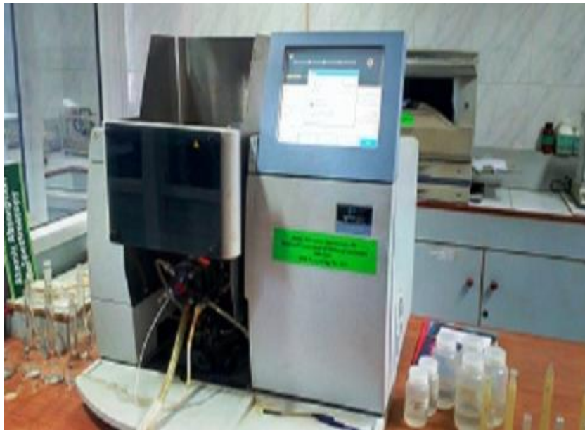
Plate 3.4: Atomic Absorption Spectrophotometer
