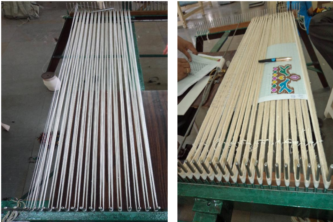
Figure 3.32. Preparation of weft.
