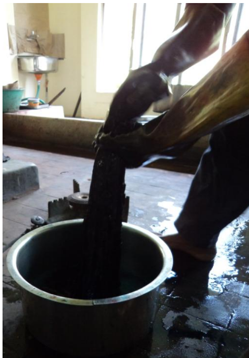
Figure 3.33. Dyeing of the yarn with Naphthol dye.
