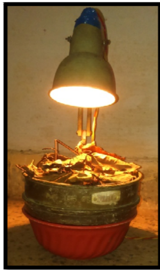
Fig. 3.2.1: Low cost Berlese funnel (Using study lamp)
