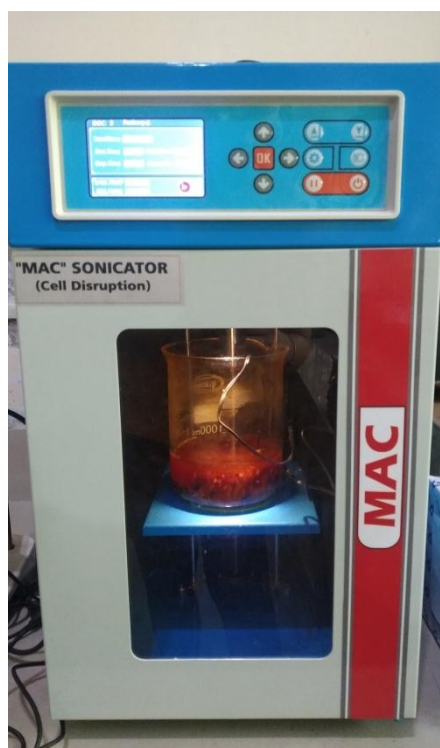
Figure 3.5: Extraction of oleoresins using ultrasonicator
