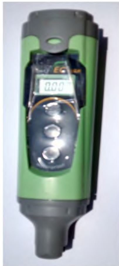
Plate 4. Milk Electrical Conductivity tester (ECO Testr®)
