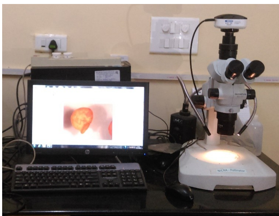
Plate. 3.2 Determination of linear dimensions by using Q-capture method
