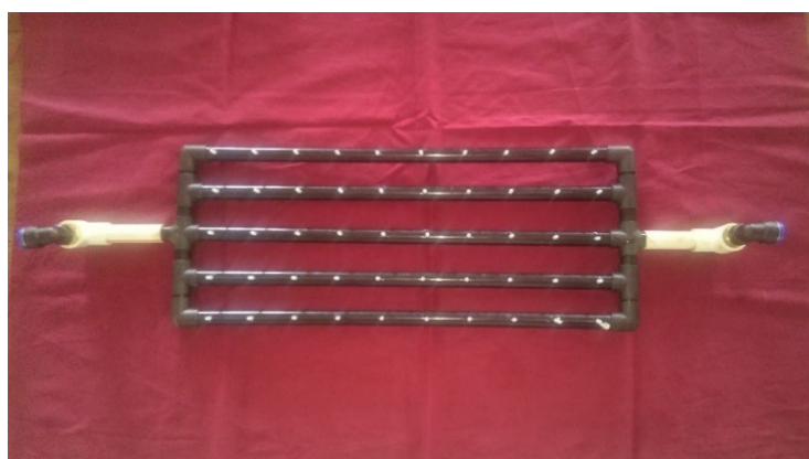
Plate. 3.5 (d) Location 4- Inlets at center on both ends
