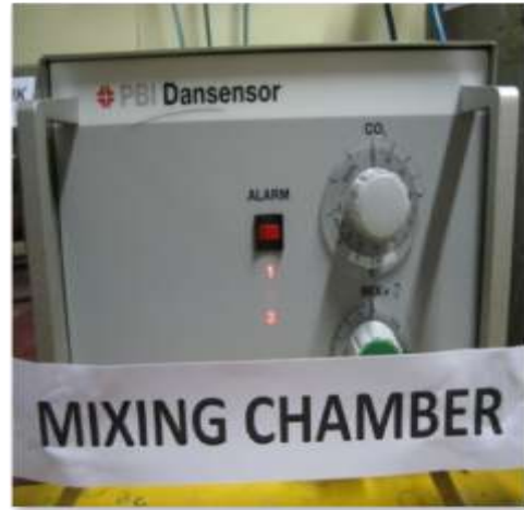
Plate 2: Gas mixing chamber
