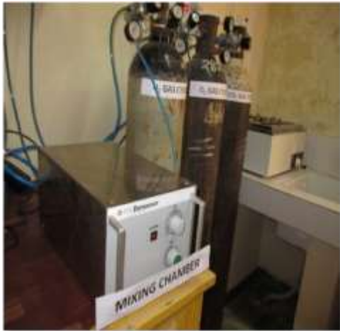
Plate 1: Gas cylinders with mixing chamber
