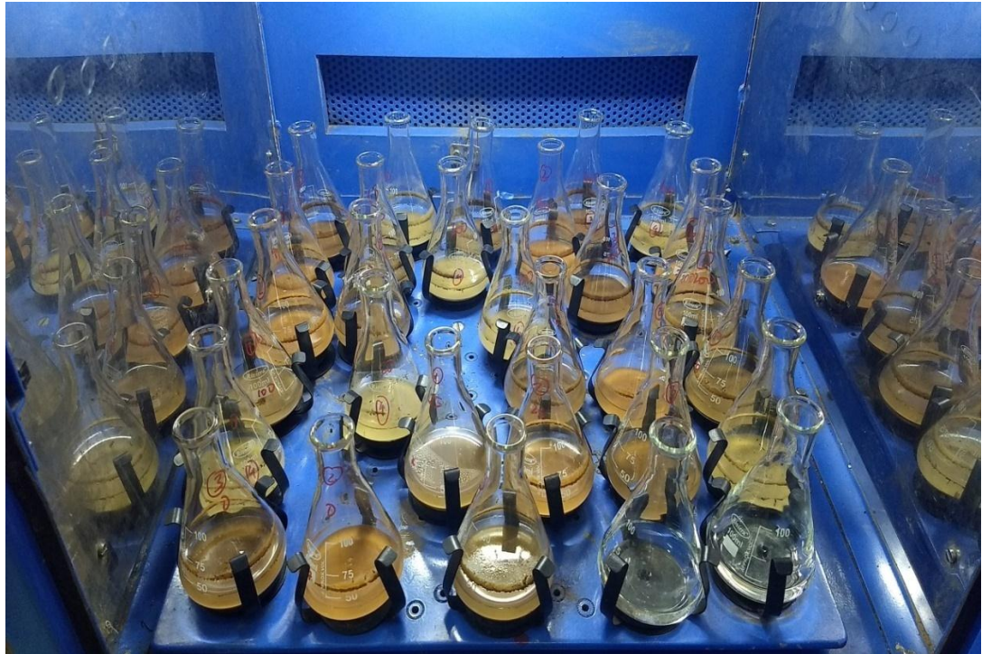
Fig. 3.4. Equilibration of soil with added P levels in 0.01 M \text{CaCl}_2 (25 ml) for 24 h.
