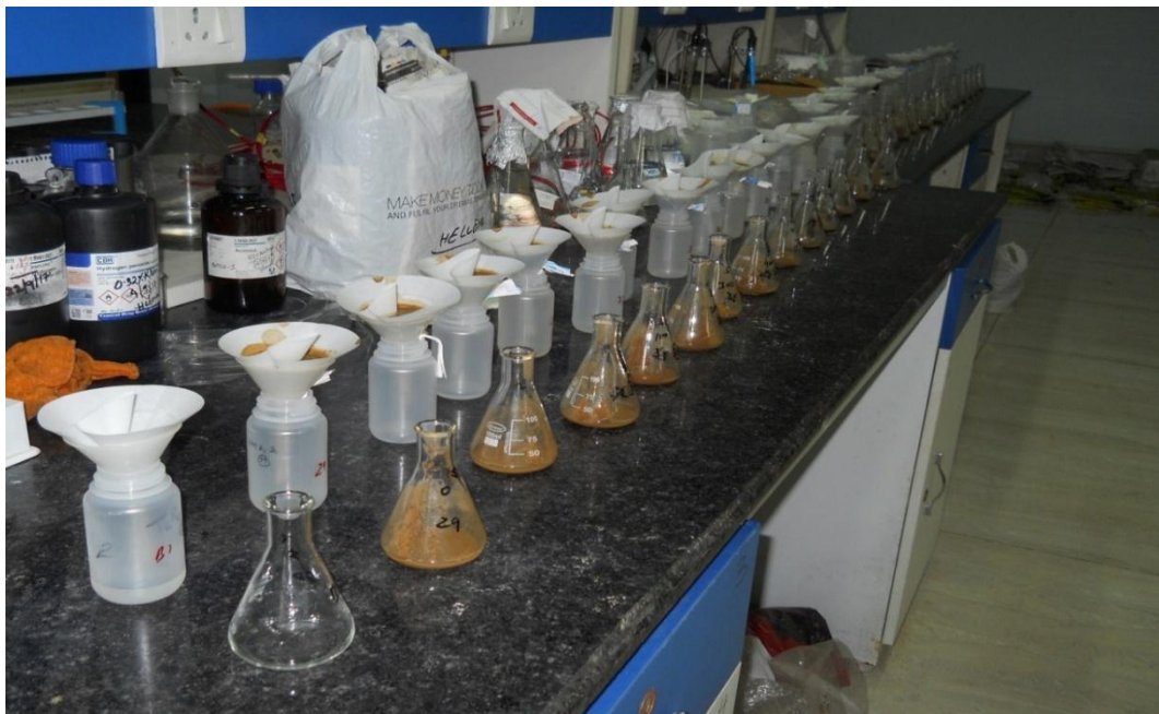
Fig. 3.5. Filtration of solution phase after equilibration with 0.01 M \text{CaCl}_2 (25 ml) for 24 h for determination of solution P content using Bray's-I method.
