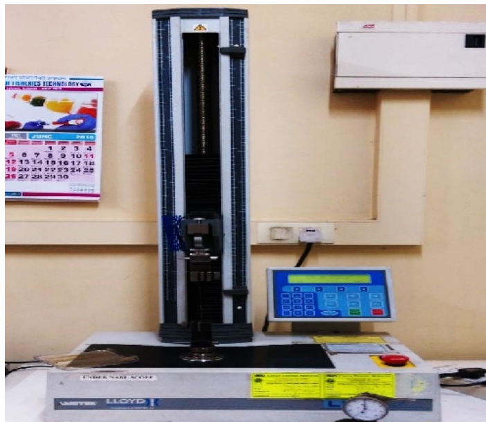
Plate 8: Measurement of mechanical properties of films
