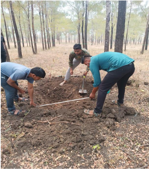
Plate 5: Preparation of pit and collection of soil samples.
