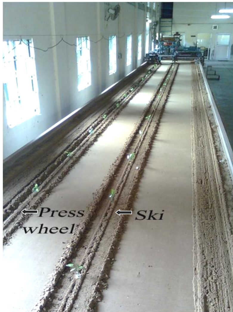
Plate 3. Testing of experimental transplanting mechanisms in soil bin
