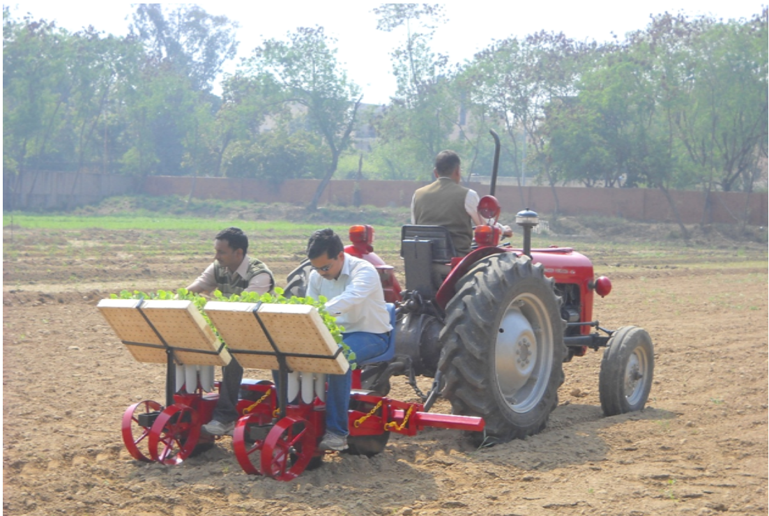
Plate 5. Field evaluation of prototype vegetable plug seedling transplanter
