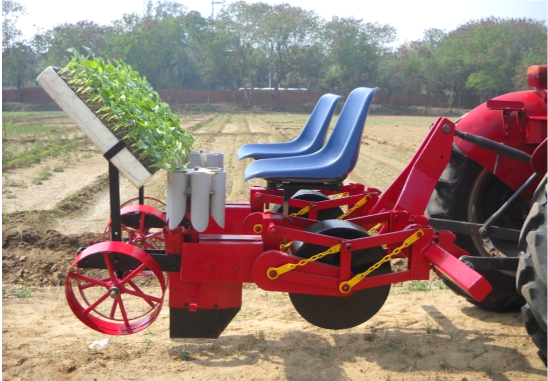
Plate 4. Tractor mounted two-row vegetable plug seedling transplanter
