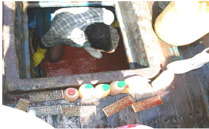
Fig.6. Cleaning of fish hold
