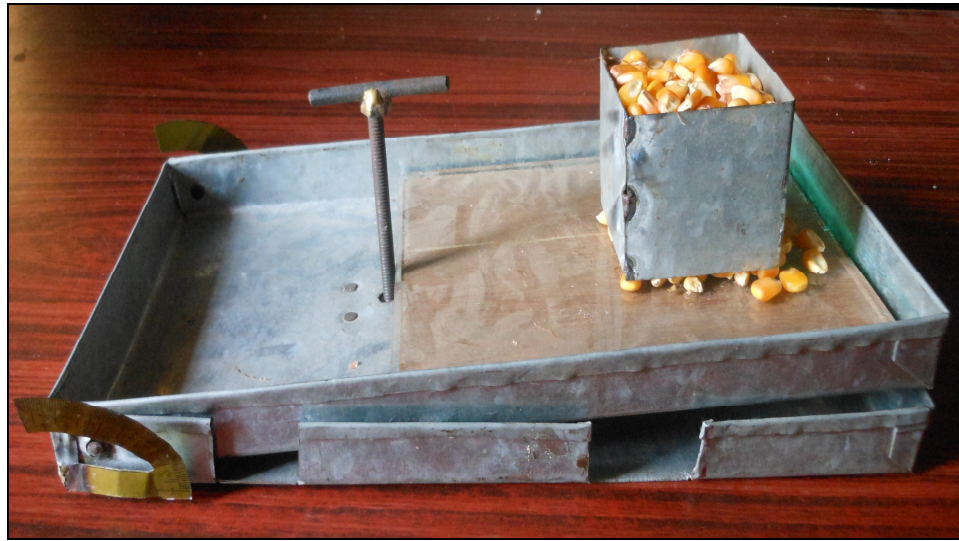
Plate 3.2. Apparatus used for measuring angle of repose.
