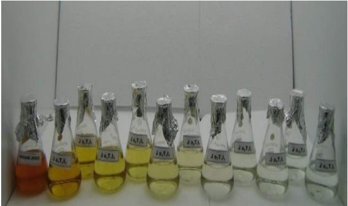
Fig 4.4a CBJ after the treatment with increasing PAC concentration from left to right at adsorption temperature of 30 °C and 30 min adsorption duration
