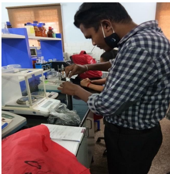
Fig. 3.18 (a) Measurement of bulk density
