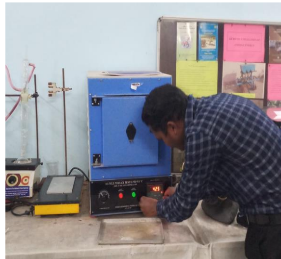
Fig. 3.17 Measurement of volatile matter
