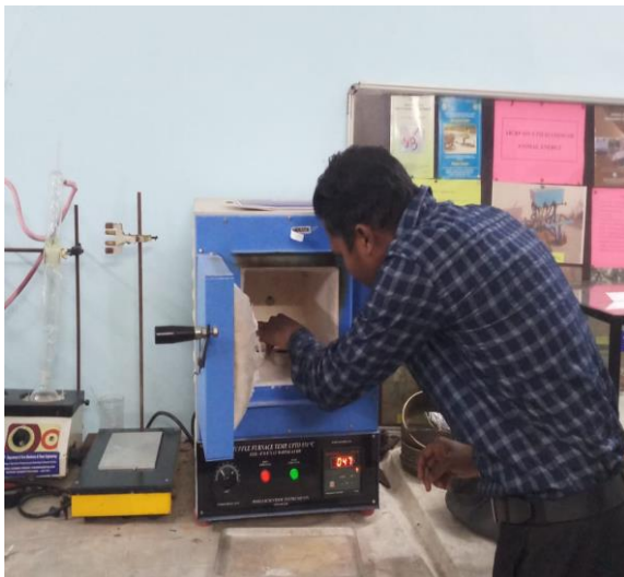
Fig. 3.16 Measurement of ash content
