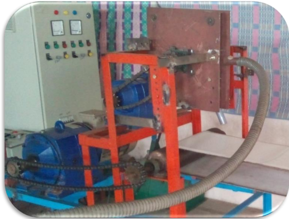
Plate 3.2 Arrangement of drive for testing of seed metering mechanism on test rig
