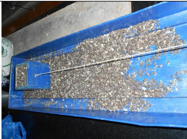
3.1c Coefficient of friction measurement between seeds
