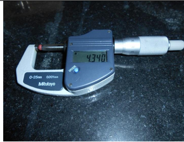
3.1a Measurement of linear dimension of seed
