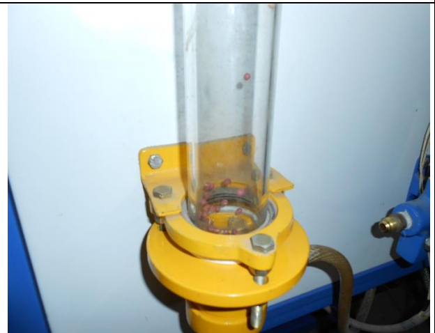
3.1d View of suspended seeds while measuring terminal velocity
