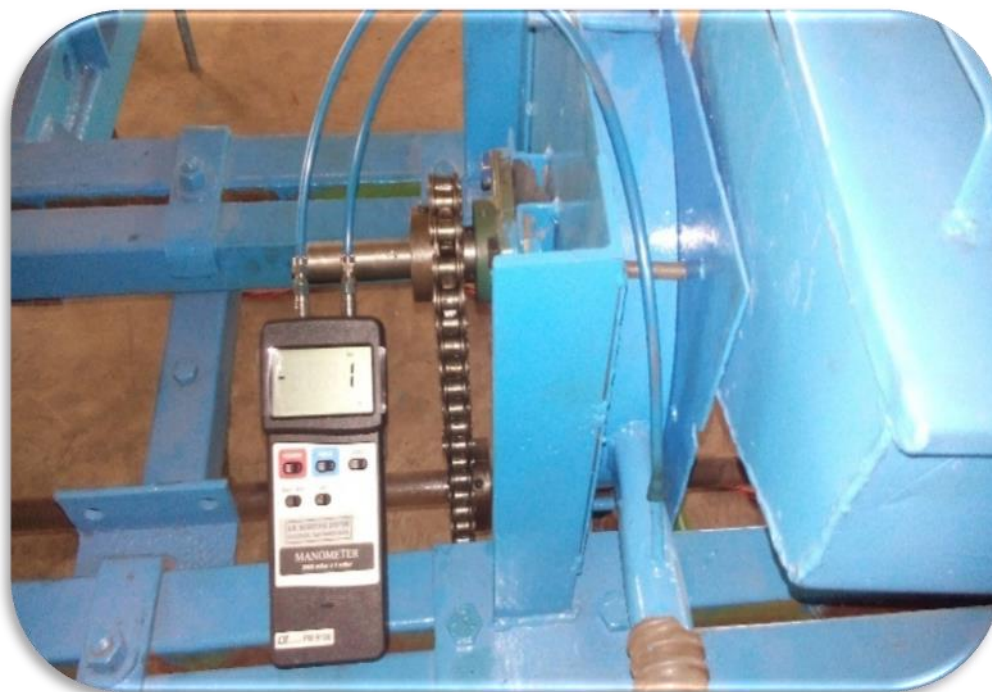
Plate 3.3 Vacuum pressure measurement by using digital manometer
