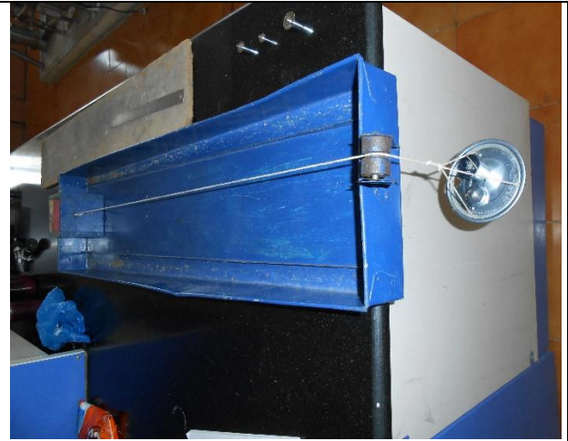
3.1b Coefficient of friction measured on MS sheet
