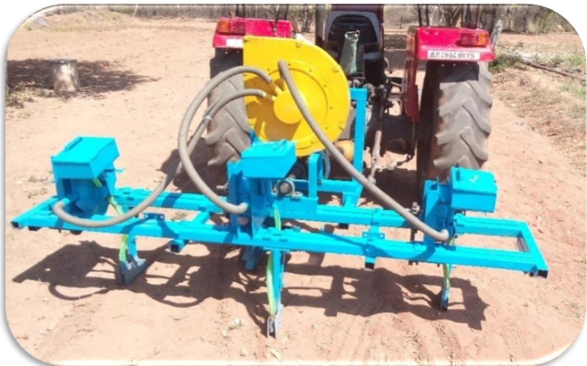
Plate 3.5(b) Rear view of pneumatic planter prototype during field evaluation
