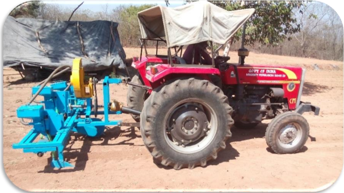
Plate 3.5(a) Side view of pneumatic planter prototype during field evaluation
