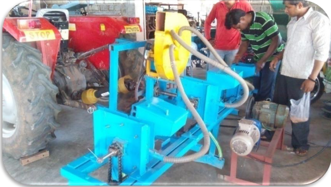
Plate 3.4 Laboratory calibration of developed pneumatic planter
