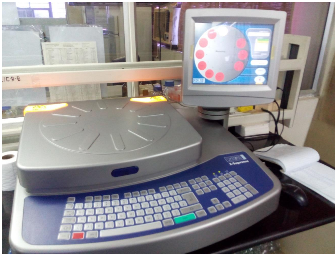
Plate 2: X- Ray Fluorescence instrument used to estimate Zn and Fe in different parts of rice grain
