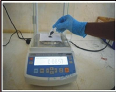
a. Weigh a small amount of soil sample (0.005- 0.015g) from the collected soil sample
