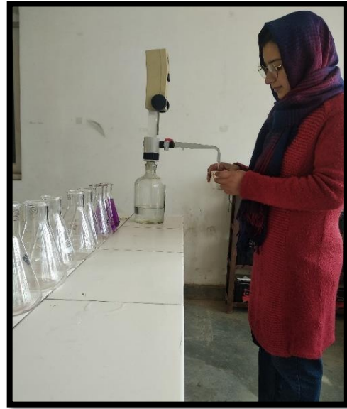
Titration with 0.01N EDTA
