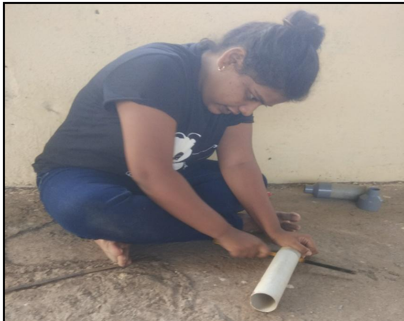
Plate 3.21 Cutting of parts for designing and development of fertigation device
