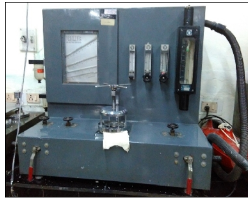
Plate 5: Shirley Air Permeability Tester
