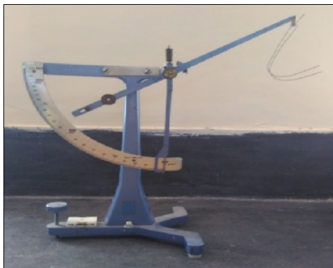
Plate 6: GSM Quadrant Balance
