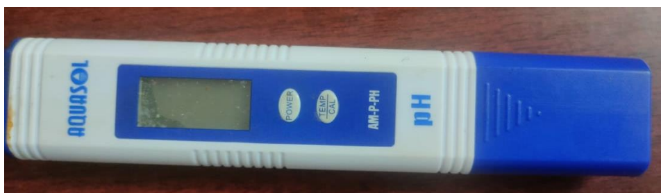
Plate 3.20 Aquasol Pen type pH meter used in the experiment
