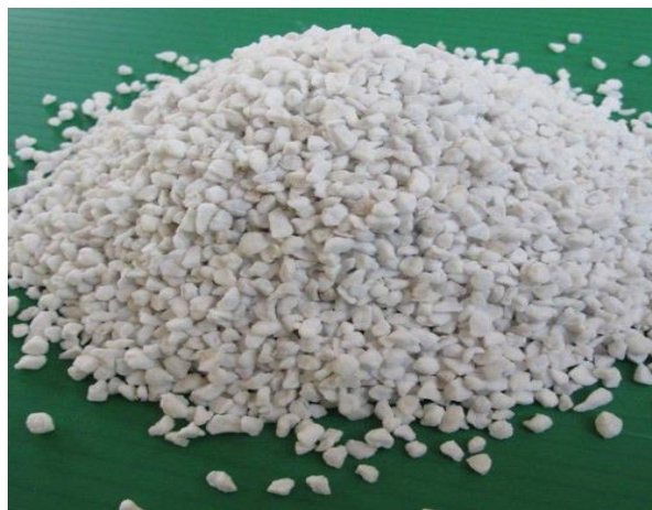
Plate 3.11 Perlite media used in the experiment.
