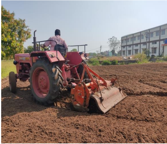
Plate 3.15 Field preparation by rotovator
