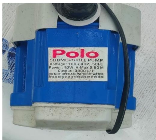
Plate 3.2 Pump used in the nutrient film technique
