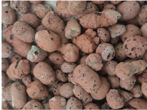
Plate 3.10 Clay balls media used in the experiment
