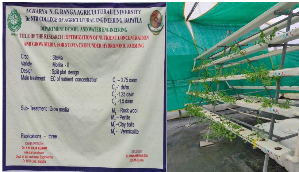
Plate 3.6 Design and layout of experiment
