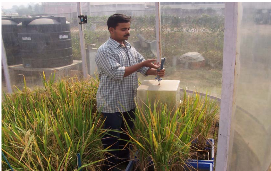
Plate 1. Gas sampling from rice soil for methane and nitrous oxide analysis.
