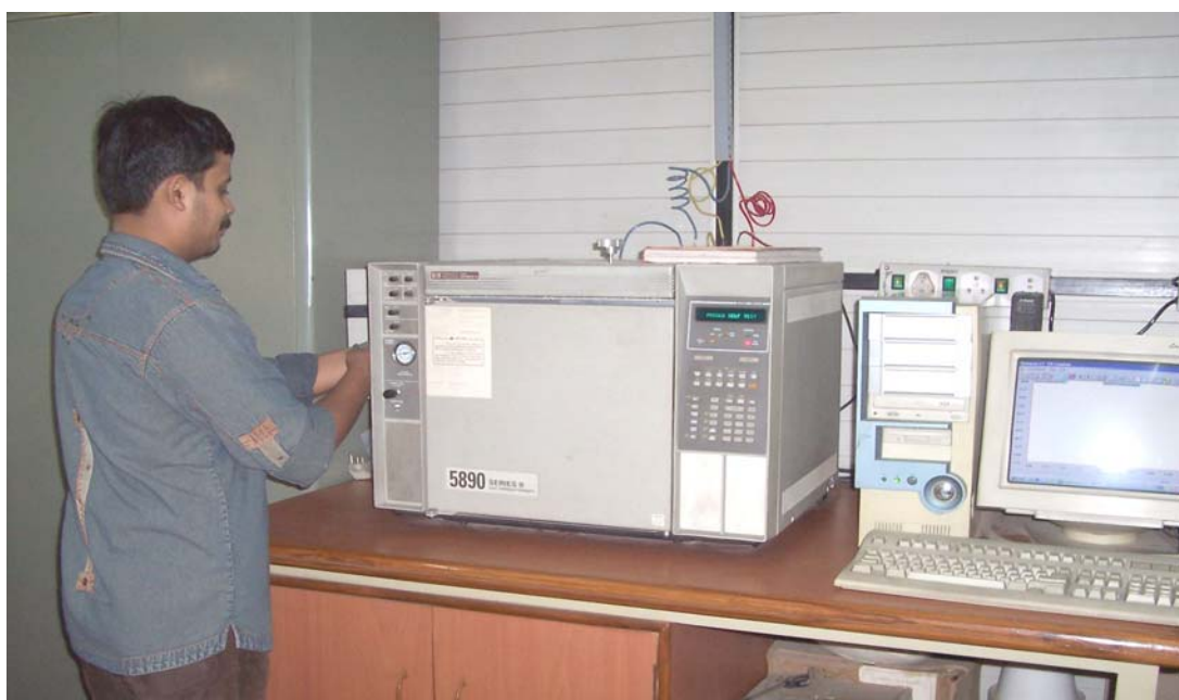
Plate 2. Analysis of gas samples for \text{CH}_4 and \text{N}_2\text{O-N} .
