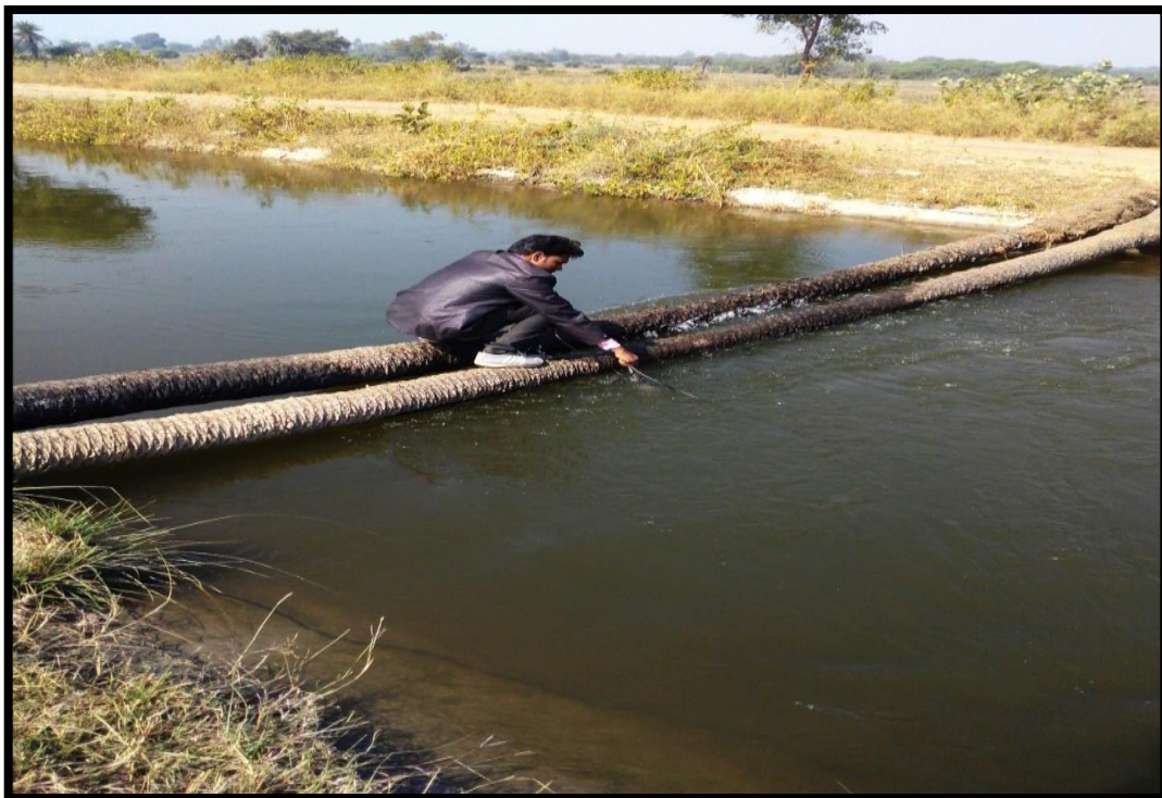
Plate 4.2 Measurement of Canal Water Flow Velocity in Middle Reach RBC
