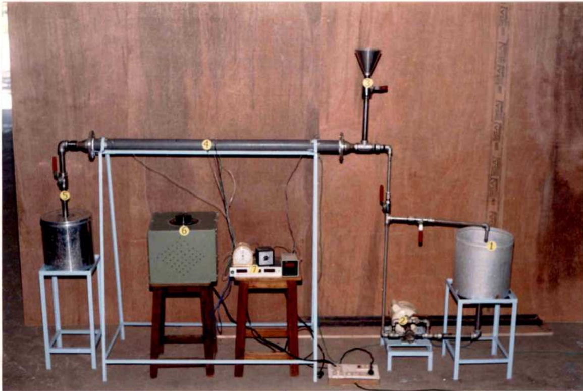
Plate 3.1 Continuous Ohmic heating System
