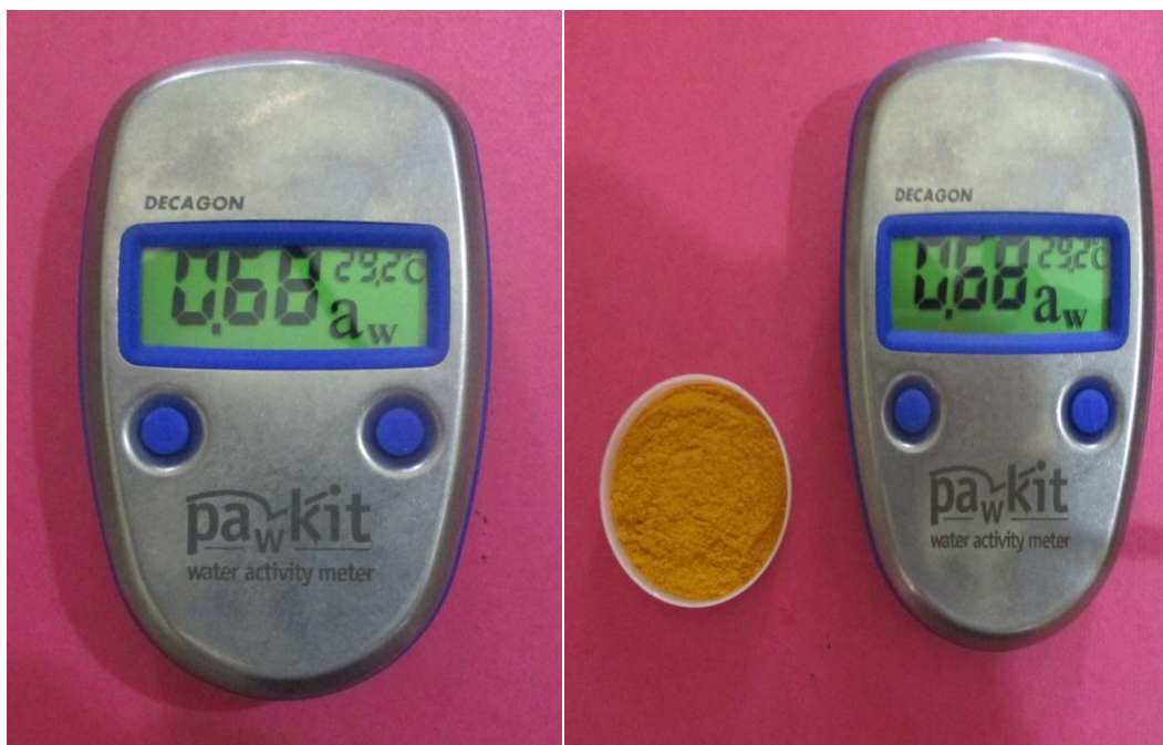
Fig. 3.8 Water activity measurement
