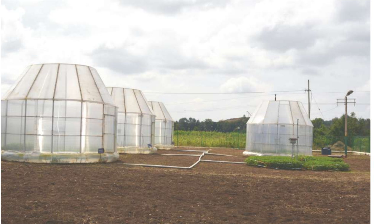
Plate 1 General view of the experimental site showing Open Top Chambers covered with poly carbonate sheets
