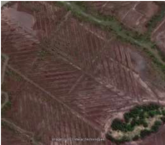
Plate 4.2: Mangrove restoration through a network of canals using fish-bone method during the years 2003 and 2022
