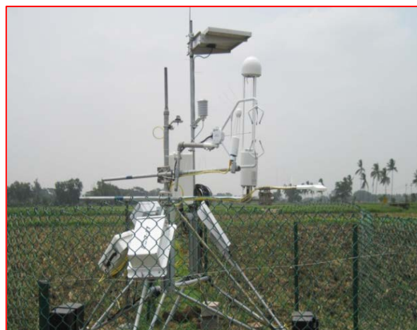
Comparison Between Eddy Covariance flux monitoring system and Closed Chamber method at CRRI, Cuttack
